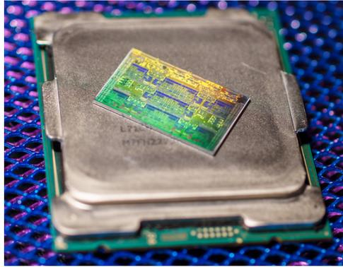
Figure 1.1: An Intel Core i7-7820X CPU (14nm node), showing the (coloured) die - the IC itself - removed from its heatsink and external casing. The die has been etched to the polysilicon layer and photographed with a reflected light microscope: for reference, it has approximately the same surface area as a one penny coin. Image reproduced from [9].
